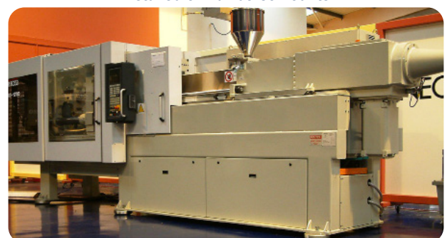
Fig. 1.2 Injection moulding machine installed on Farrat Isomounts
