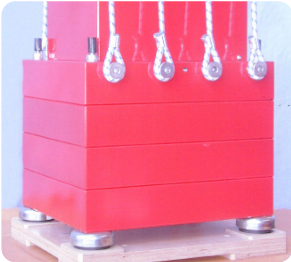
Fig. 2.1 Shock testing machine installed on Farrat Isomounts
