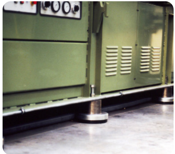
Fig. 2.4 Injection Moulding Machine installed on Farrat Isomounts
