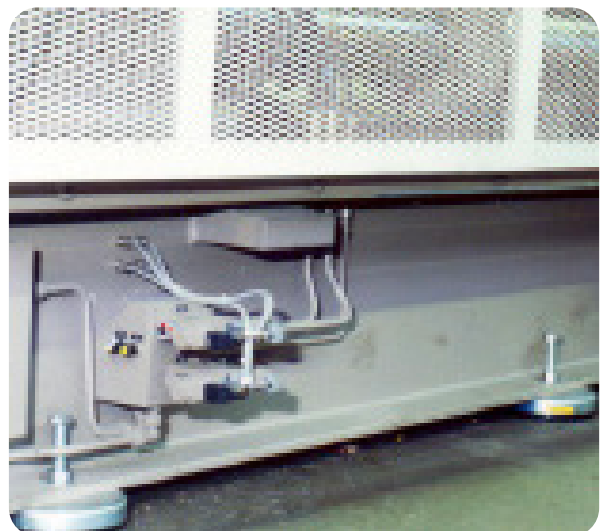
Fig. 2.6 Injection Moulding Machine installed on Farrat Isomounts
