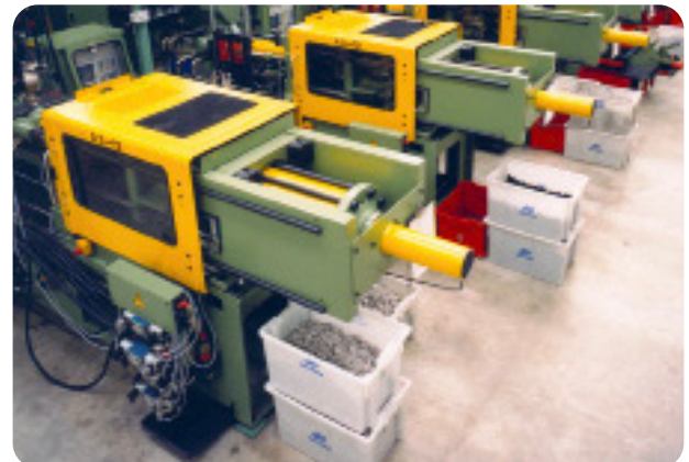
Fig. 1.2 Injection moulding machine installed on Farrat Isomounts
