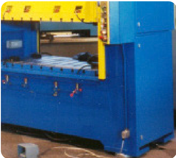
Fig. 2.3 Rhodes Power Press installed on Farrat Isomounts
