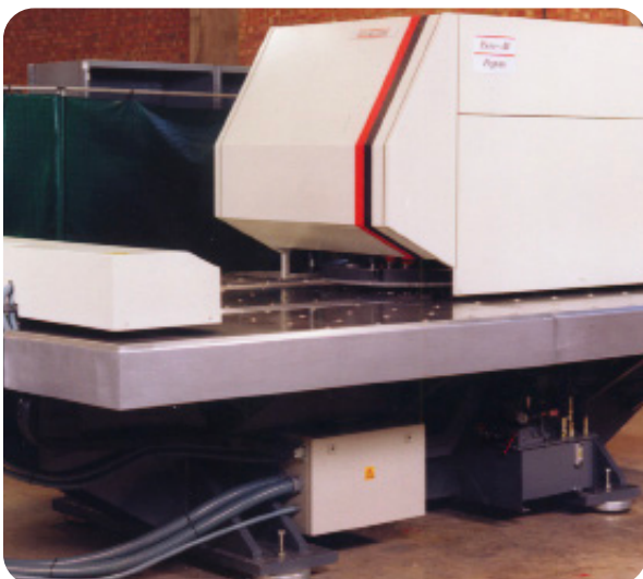
Fig. 2.5 Turret Punch installed on Farrat Isomounts
