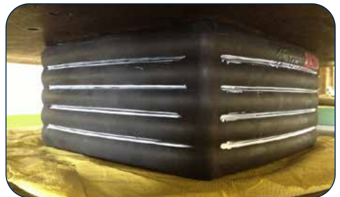
Fig 8.2 Five-Layer LNR Bearing Under Compression Load
