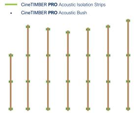
CineTIMBER **PRO** acoustic isolators can be designed to match any baseplate and washer quantity combination (subject to load limits). See the CineTIMBER brochure for further information.
