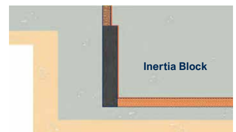
Fig 6.4 Type 3 For inertia blocks needing full area base support. See full area materials on Page 18
