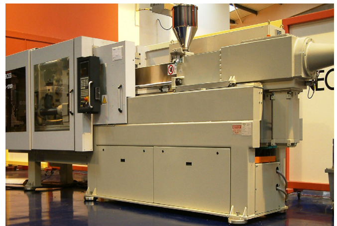
Fig. 1.2 Injection moulding machine installed on Farrat Isomounts
