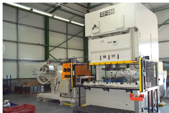
Fig. 1.1 Power Press installed on Farrat Isoblocs
