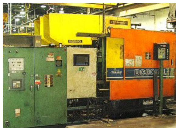
Fig. 1.2 Die Casting machine installed on Farrat Isoblocs
