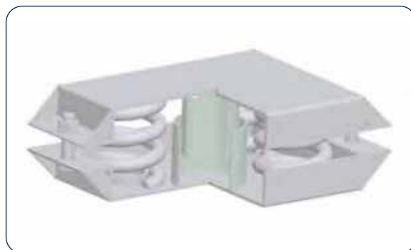
Fig 7.15 FSLV Combined Spring/Damper Unit
