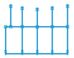
**CineSTEEL PRO** acoustic isolators can be designed to match any baseplate and washer quantity combination (subject to load limits). See the CineSTEEL brochure for further information.
