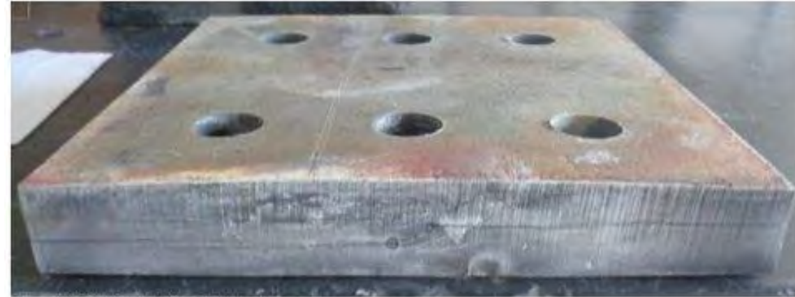
Figure 17: TBF Coated Post-Firetest
