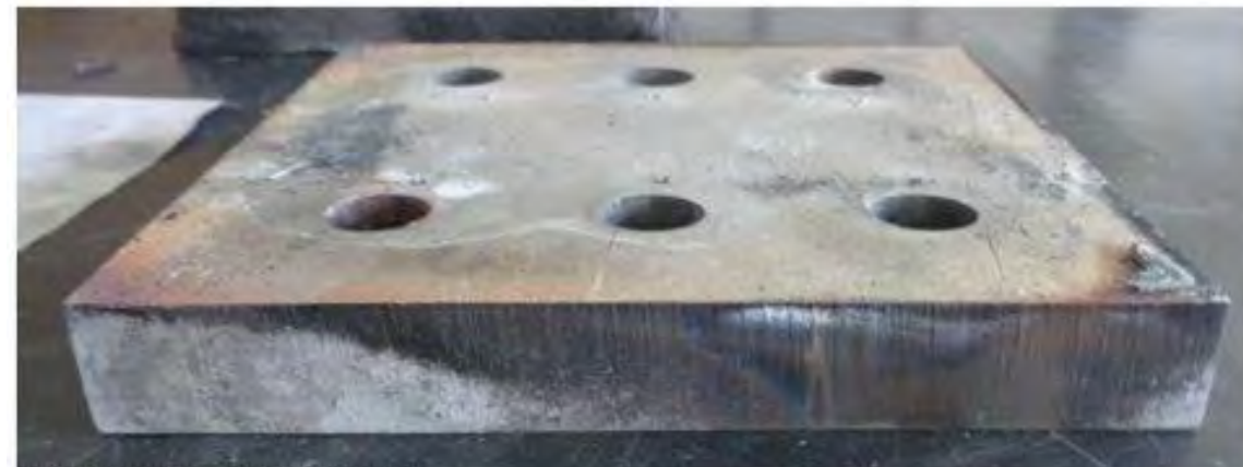
Figure 18: TBF Uncoated Post-Firetest
