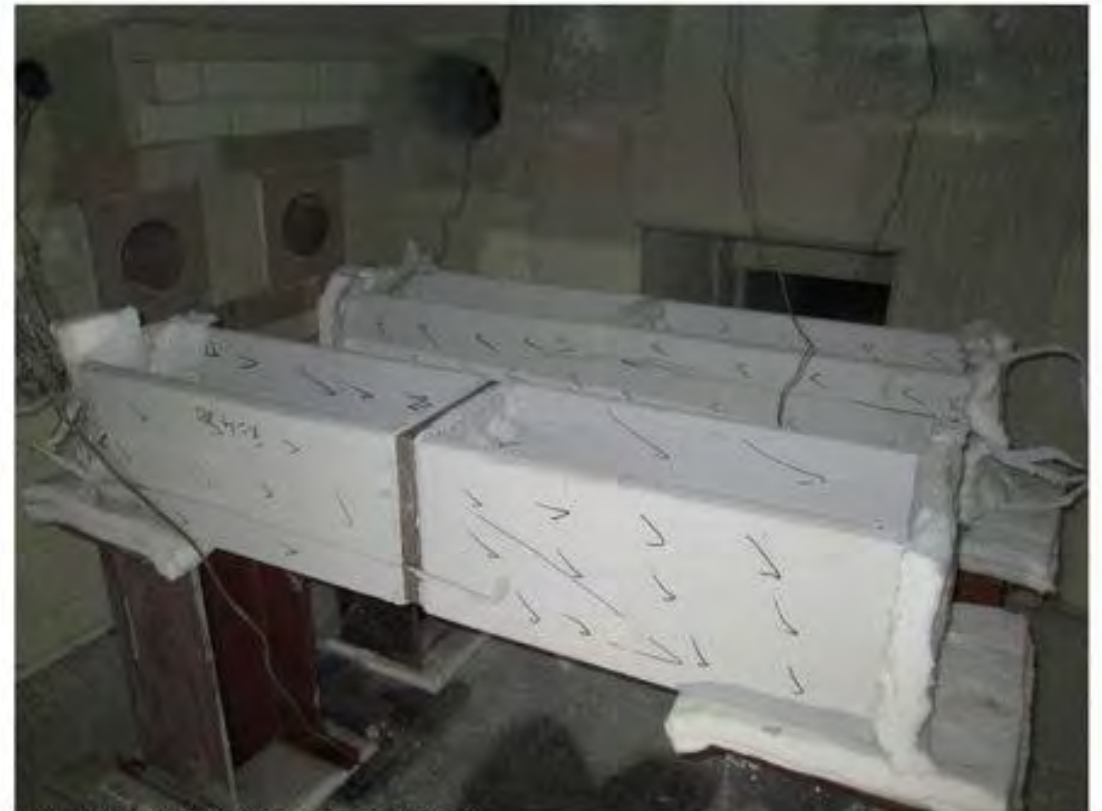
Figure 5: TBF Sections Pre-Firetest
