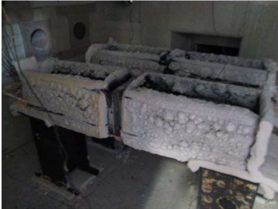
Figure 8: TBF Sections Post-Firetest
