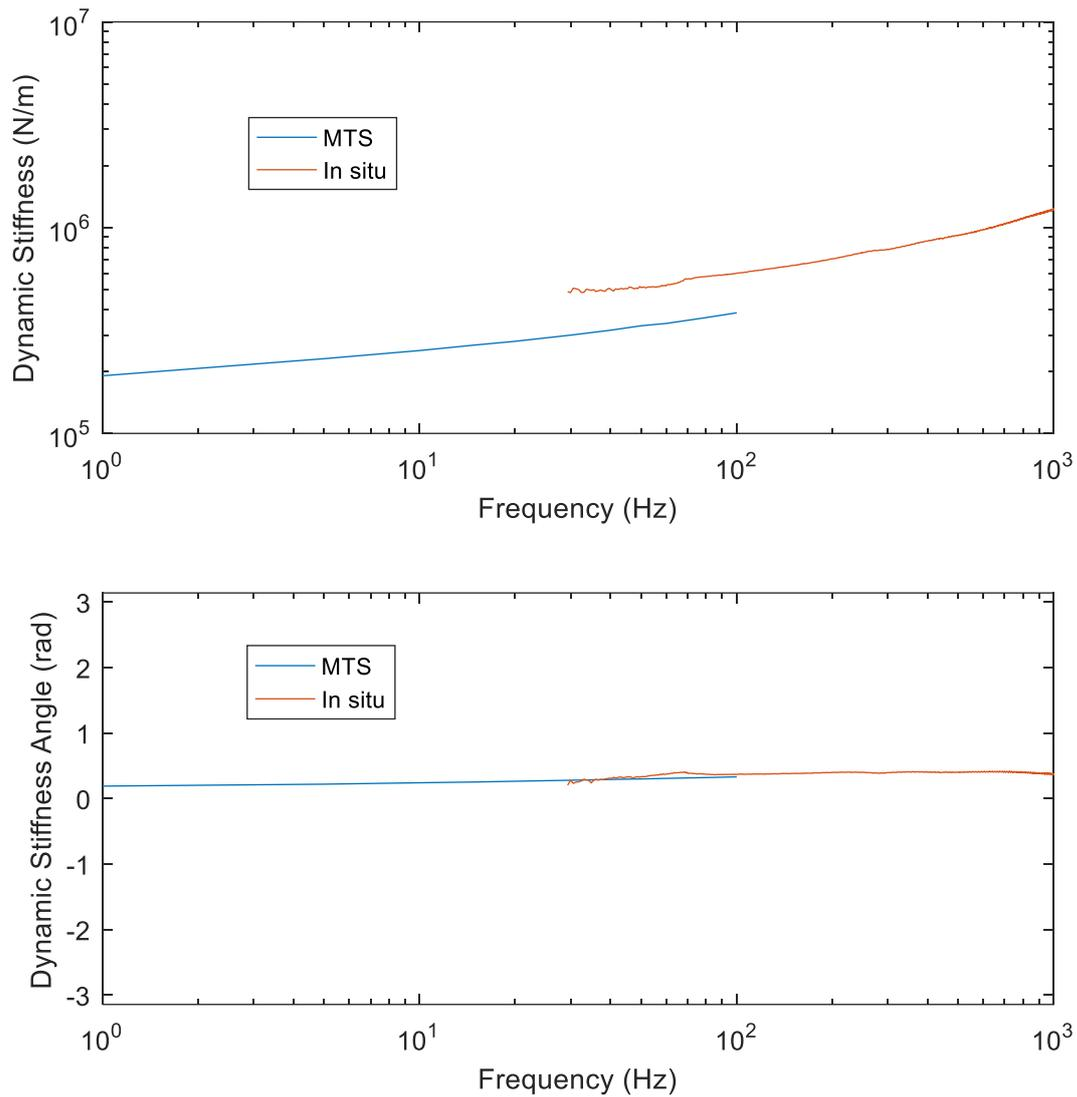
Figure 5: Dynamic stiffness of VIDAM isolator measured using the *in situ* Mass-isolator-mass procedure (red) vs. using Dynamic compression (blue) in both terms of magnitude (top) and phase (bottom).
