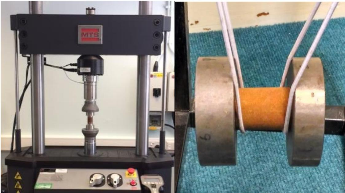
Figure 4: dynamic compression (left) and *in situ* (right) isolator characterisation experimental setups
