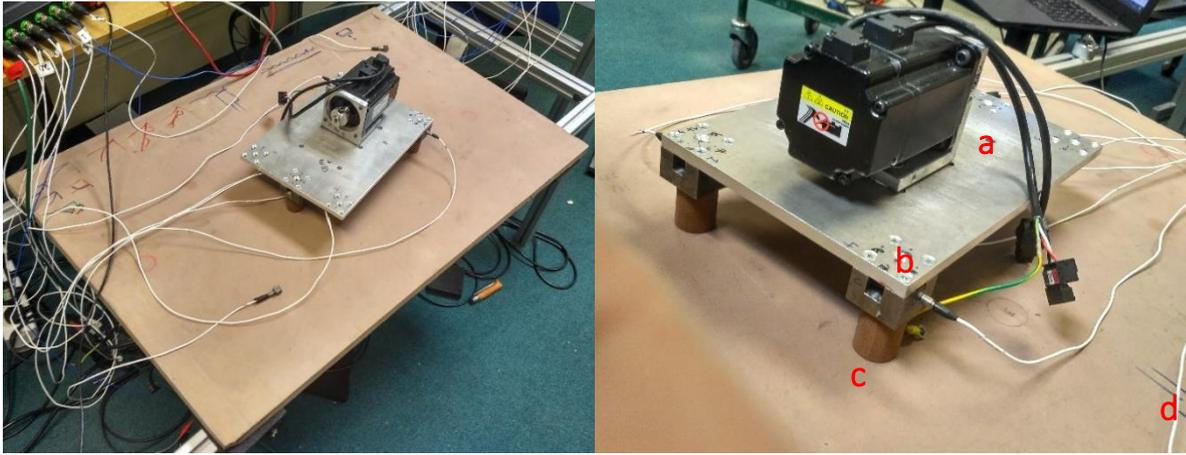
Figure 6: Left: Coupled Source-Isolator-Receiver assembly experimental setup. Right: Closer view of the assembly identifying the different interfaces (a-d) in red font.
