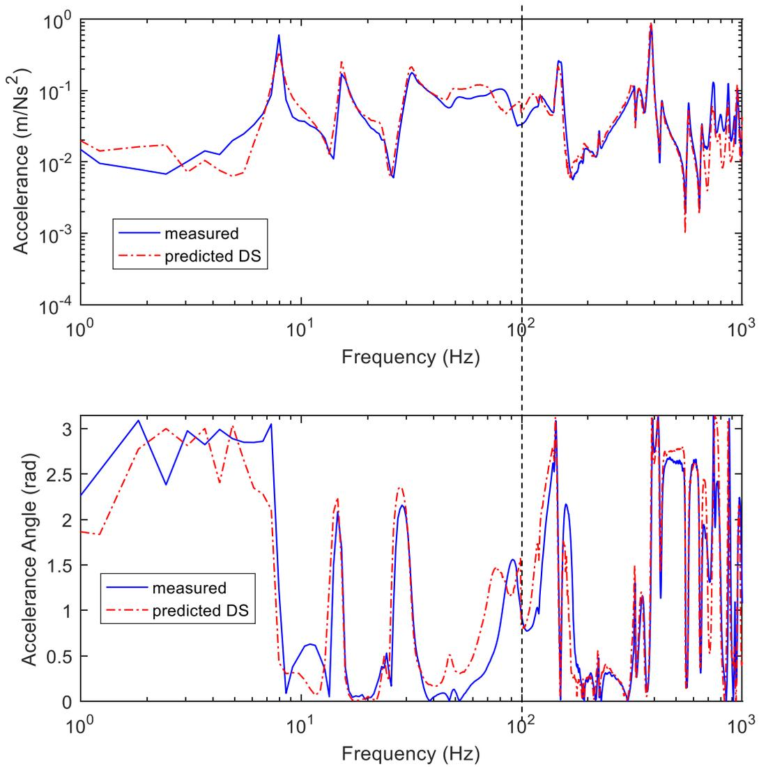
Figure 7:  $A_{C,d}$  accelerance obtained in the coupled measurement (blue) vs prediction using the dynamic sub-structuring method (red-dashed) in terms of magnitude (top) and phase (bottom). Black dashed line divides the isolator characterisation between MTS (below 100Hz) and *in situ* methods.
