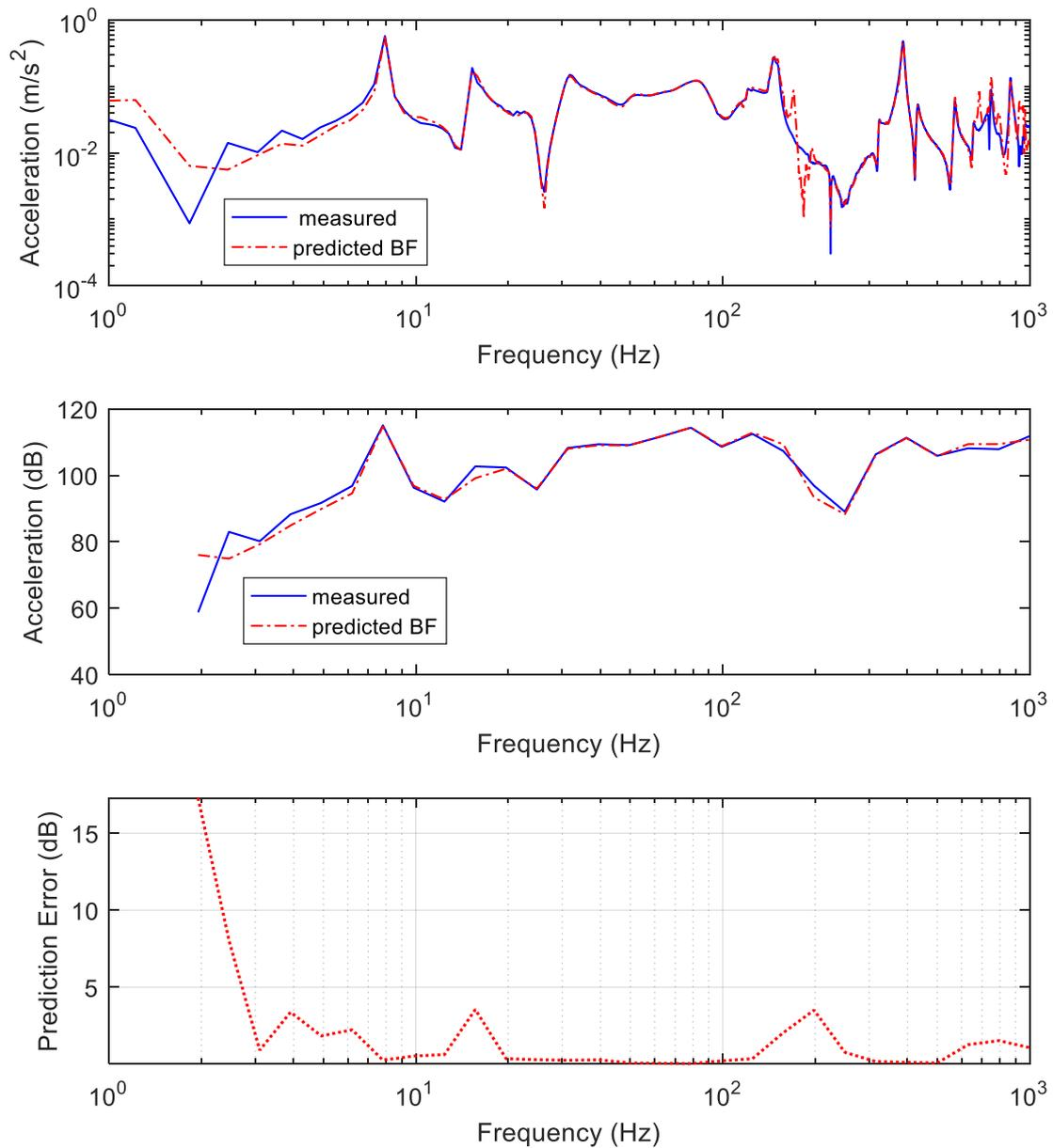
Figure 3:  $a_{c,d}$  acceleration obtained in the coupled measurement (blue) vs prediction using the blocked force method (red-dashed) in narrow band frequency (top) in  $m/s^2$  and per third octave band (middle) in decibels (ref.  $1\mu m/s^2$ ). Bottom: error between prediction and *in situ* obtained coupled acceleration (dB) in third octave bands.
